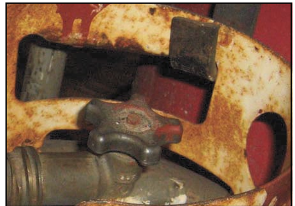
The propane tank used in this workplace incident (star-shaped handle as shown here) was not equipped with an excess flow valve.
